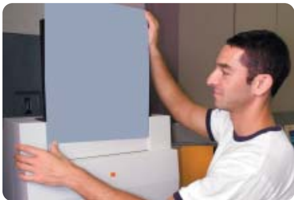
Nunzio Esposto, RT(T), inserts exposed media into the Kodak 2000RT CR system for scanning.
